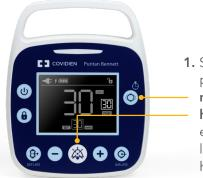
1. Simultaneously press and hold the mute and pressure hold buttons after enabling time-limited pressure hold function.
