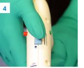
Pull and hold the blue lock switch button in the back position.
