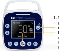
Simultaneously press and hold the mute and pressure hold buttons after enabling time-limited pressure hold function.
