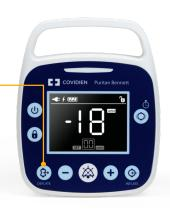
**Tip:** When the cuff is deflated, the indicator for the target pressure setting will appear gray and the pressure display is negative (usually <-10 cmH<sub>2</sub>O).
